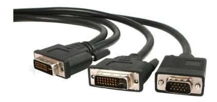
The DVIVGAYMM6 6-foot DVI-I (male) to DVI-D (male) and HD15 VGA (male) video splitter cable lets you connect a DVI-D monitor as well as a VGA monitor to a single DVI-I video card port.
