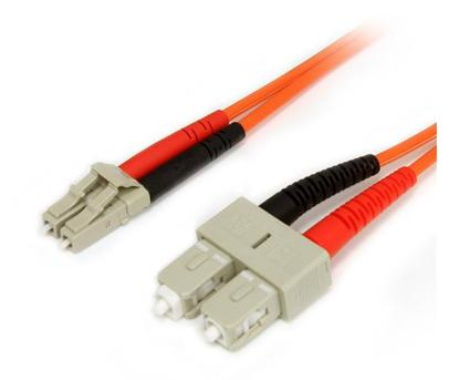
The FIBLCSC2 2-meter (6.6ft) Multimode 62.5/125 Duplex Fiber Patch Cable is terminated with one LC (male) connector and one SC (male) connector, to provide the necessary connection between fiber networking devices for high-speed, long distance networks.
