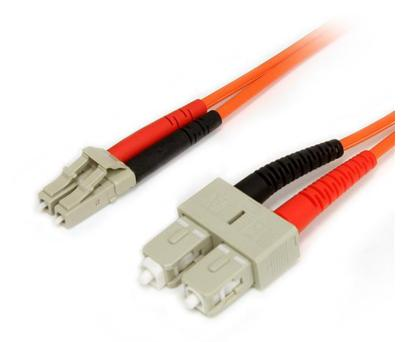
The FIBLCSC3 3-meter (10ft) Multimode 62.5/125 Duplex Fiber Patch Cable is terminated with one LC (male) connector and one SC (male) connector, to provide the necessary connection between fiber networking devices for high-speed, long distance networks.
