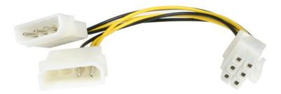
This 6in LP4 to 6 Pin PCI Express Video Card Power Adapter converts a standard LP4 power connector on your existing power supply to a 6 pin PCI Express video card power connector, allowing you to install a PCIe graphics card without having to upgrade the computer power supply.
