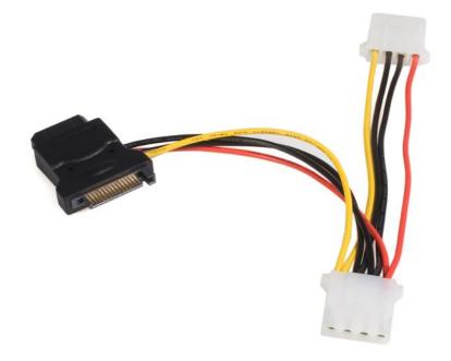
The LP4SATAFM2L SATA to LP4 Power Cable, lets you power an IDE (LP4-connected) drive using a SATA power connector from the computer power supply. The adapter features two additional LP4 power connectors, offering the versatility to connect two additional (LP4 connected) drives (CD/DVD-ROM, HDD, etc.) using the same single connection to the computer power supply.
