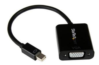
The MDP2VGA2 Mini DisplayPort to VGA converter enables you to connect your Mini DisplayPort video source (Laptop, Macbook®, Ultrabook etc.) to a VGA monitor or projector, saving the expense of upgrading to a Mini DisplayPort compatible display. The mDP adapter is the perfect accessory for your Microsoft Surface™ Pro 4, Surface Pro 3, Surface 3, Surface Pro 2 or Surface Book.
