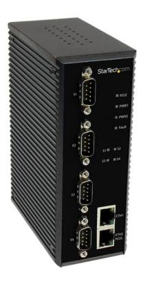
The PoE-powered NETRS42348PD 4-Port Industrial Serial Device Server lets you remotely manage up to four industrial RS232/422/485 serial devices over a local or wide area network (LAN/WAN), with redundant power inputs and dual 10/100Mbps Ethernet ports.
