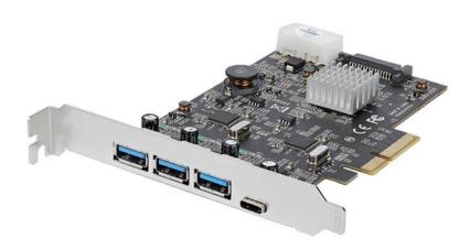
This USB 3.1 PCIe card lets you add three USB Type-A ports and one USB Type-C port to your computer, through a PCI Express slot. It makes it easy to upgrade your PC to the faster speed of USB 3.1 (10Gbps) so that you can access newer peripherals at twice the speed of traditional USB 3.0 (5Gbps) cards.
