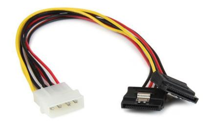
The PYO2LP4LSATA LP4 Molex to Dual Latching SATA power splitter cable features two Serial ATA female power connectors and one LP4 male connector - a reliable solution that enables you to power two SATA drives using a single LP4 connection to the computer power supply.
