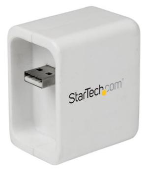
This Wireless N travel router lets you create a portable wireless hot-spot from a wired network connection or an existing wireless network, to share with all of your Wi-Fi® enabled devices, including tablets, laptops, Ultrabooks<sup>™</sup>, or smartphones.
