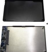
2. Place the 2.5" SATA drive into the half of the enclosure that contains the SATA connector, and slide the drive onto the SATA connector.
