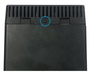
2. Slide the "front panel" upward toward the top of the enclosure.
