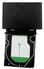
Place the front panel back on by placing it over the drive bay, and sliding it into place.
