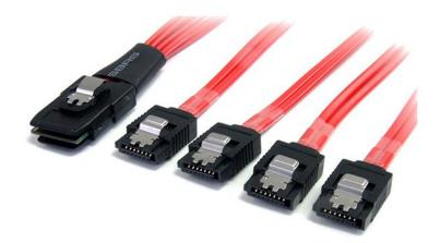
The SAS8087S450 SFF-8087 to 4x SATA SAS cable features one 36-pin plug (SFF-8087), which fans out to four SATA 7-pin receptacles, providing a reliable solution for connecting up to four SATA HDDs to a SAS controller or backplane.
