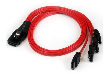
The SAS8087S4R50 SFF-8087 to 4x SATA Reverse cable features one 36-pin plug (SFF-8087), which fans out to four SATA 7-pin receptacles, providing a reliable solution for connecting a Mini SAS backplane to a SAS / SATA RAID controller or motherboard.
