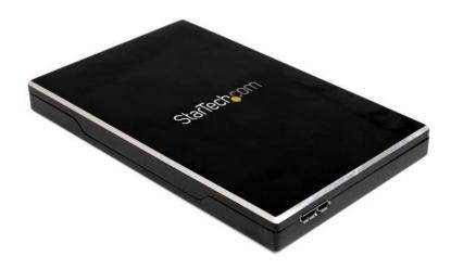
The SAT2510BU32 2.5-inch SuperSpeed USB 3.0 SATA Hard Drive Enclosure turns a normal 2.5-inch SATA hard drive (HDD) or solid state drive (SSD) into a portable, external hard drive.
