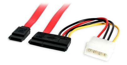
The SATA18POW SATA Data and Power Cable features a combination 22-pin SATA receptacle data and power connector as well as an Molex (LP4) power connector and SATA receptacle data connector, allowing you to create a conventional Serial ATA data connection to a computer while powering the drive through an LP4 connection to the computer power supply.
