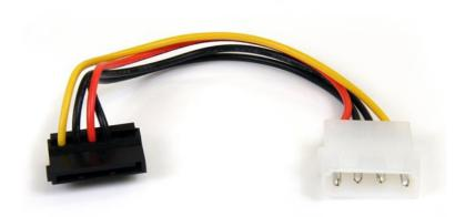
This 6-inch 4-Pin (LP4) Molex to Right Angle SATA power adapter features one 4-Pin Molex (LP4) male connector and one (female) right angle SATA power connector, allowing you to power a Serial ATA hard drive from a conventional LP4 connection, eliminating the need to upgrade the computer power supply for compatibility with the SATA hard drive.
