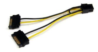
The SATPCIEXADAP SATA to PCI Express Video Card Power Adapter Cable features a 6-pin PCI Express (male) power connector as well as two 15-pin SATA (male) power connectors, providing a cost-effective way to connect a PCIe video card to Serial ATA power connectors provided by the computer power supply, and eliminating the need to upgrade the power supply for the sake of video card compatibility.
