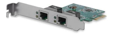
The ST1000SPEXD4 PCI Express Dual-Port Gigabit Network Card lets you add two gigabit Ethernet ports to a client, server or workstation through a single PCIe slot. Each port provides 10/100/1000 Mbps capable Ethernet and is fully compatible with IEEE 802.3/u/ab standards.
