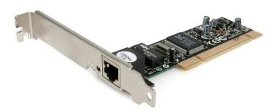
This 1 Port PCI Fast Ethernet Network Adapter Card offers a reliable, cost-effective Ethernet network connection. Delivering a simple connection to 10/100Mbps Ethernet networks, the NIC features auto-negotiation that senses speed and duplex capabilities of connected devices and full duplex support for data transfer rates up to 200Mbps.
