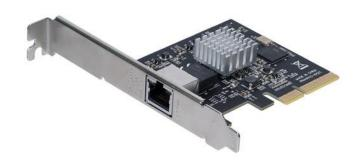
This 5-speed network adapter card offers versatile and cost-efficient network connectivity. It lets you add an Ethernet port to your server or desktop computer and access your network at multiple speeds: 10G, 5G, 2.5G 1G and 100Mbps.
