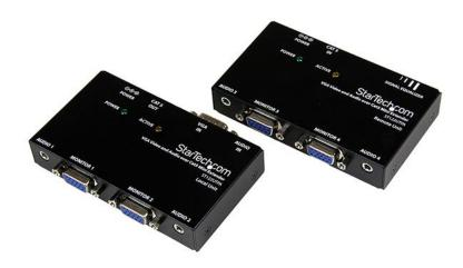
The ST122UTPAGB VGA Video Extender over Cat 5 with Audio allows up to 4 (2 local and 2 remote) monitors to be connected to a single PC. The video signal and corresponding audio are sent to the remote unit over standard 4 pair Category 5 or better (Cat 5e recommended) UTP cable, supporting extended video distances of up to 150m / 500ft.
