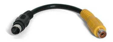
This S-Video to Composite Video Adapter features a 4-pin mini-DIN S-Video Male connector and an RCA female connector, allowing you to connect a device with S-Video output to a device with RCA Composite Video input.
