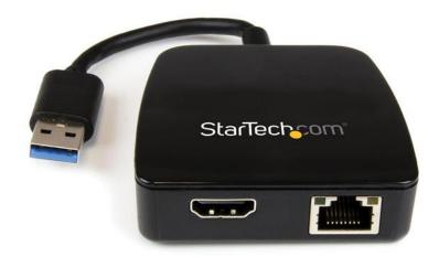
The USB31GEHD USB 3.0 Mini Docking Station Adapter lets you add Gigabit Ethernet and HDMI® connection ports to your Ultrabook™, laptop, or desktop through a single USB 3.0 host, giving you two connectivity ports that aren't always available on modern mobile computers.
