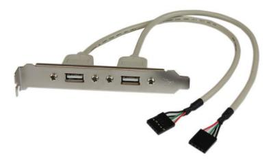
The USBPLATE 2 Port USB A Slot Plate converts the USB pins from most AT style Pentium (and newer) motherboards to 2 standard USB A-Style ports. The plate can be mounted on the rear panel of a computer case, adding two USB A female ports for simple connection to USB peripheral devices.
