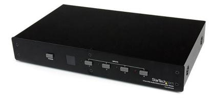
The VS410RVGAA 4 Port VGA Video Audio Switch with RS232 control lets you switch between four separate VGA signals, as well as the corresponding audio, for output to a single display or projector at resolutions up to 1920x1200 (PC) or 1080p (HDTV).
