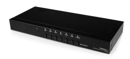
The VS721MULTI Multiple Video Input to HDMI® Switcher enables users to switch between 7 different audio-video sources to a single HDMI-equipped display.
