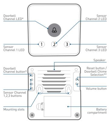
\* The Doorbell channel is reserved for Doorbell units (separate purchase required) and can only be used to pair Doorbell units with the Gate Alert system.
