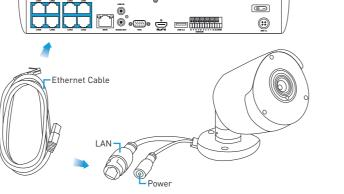
Please note: The power connector is provided as an alternative power option if required. Your NVR will provide power over the Ethernet cable when connected and a separate power adapter is not required.
