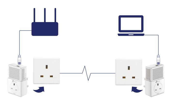
Powerline adapters and extenders must be deployed in a set of two or more.
