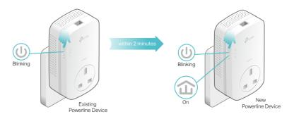
**3.** Relocate the new powerline adapter to the place where wired Internet access is needed.
