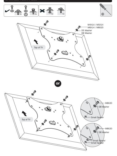
**Note:** Firmly secure the VESA plate to the display using the appropriate screws, washers and spacers (if necessary).
