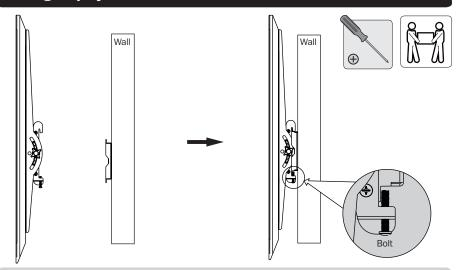
Using an assistant or mechanical lifting equipment, hook the display with attached adapter brackets over the top of the mounted wall plate. Tighten the two screws on the bottom of the adapter brackets to secure the unit.
