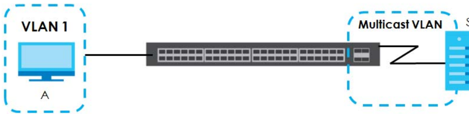
Figure 126 MVR Multicast Television Example
