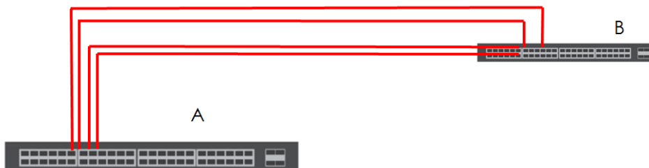
Figure 88 Trunking Example - Physical Connections
