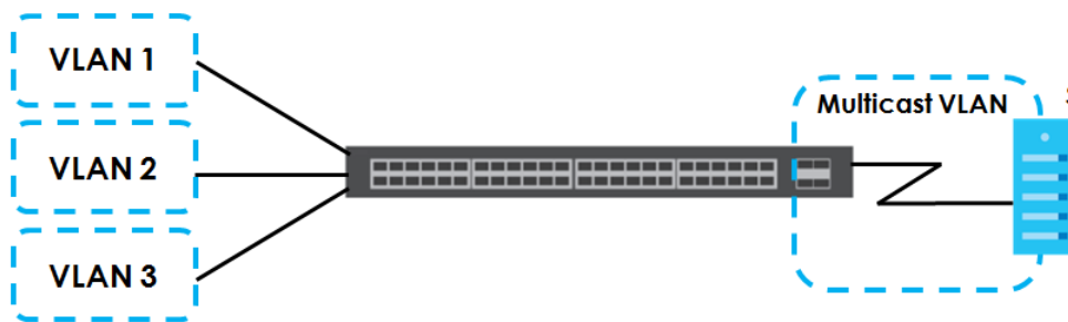
Figure 125 MVR Network Example
