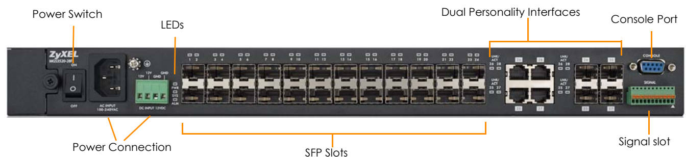
Figure 8 MGS3520-28F Front Panel: AC/DC Model
