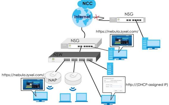
You can check the system settings via the Web Configurator, the ZON (Zyxel One Network) utility and the console port.
