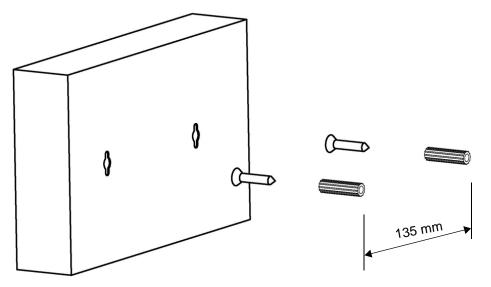
The NSW should be wall-mounted horizontally. The NSW's side panels with ventilation slots should not be facing up or down as this position is less safe.
