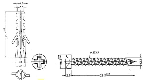
Figure 11 Masonry Plug and 3.5 mm Self-Tapping Screw
