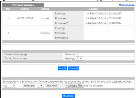
Type the path and file name of the firmware file you wish to upload to the Switch in the **File Path** text box or click **Browse** to locate it (Firmware upgrades are only applied after a reboot). Click **Upgrade** to load the new firmware.
