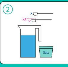
Add 2g of table salt - that's a flat measure using the measuring spoon provided. No more or less as this affects the electrolysis. If too much salt is added, rinse out the jug and start again. Do not use rock
