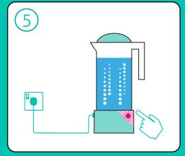
Place the jug on its base. The base will beep once and white button remain lit. Activate the solution by pressing the button once. After 3 seconds the base light will flash and beep, the jug will light up blue and microbubbles appear as electrolysis begins.
