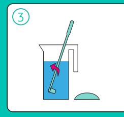
Stir the solution at least 8 times in the centre of the jug to fully dissolve the salt. The salt acts as an electrolyte and if it accumulates on the electrode the product will not work. Place the lid on the jug, and wipe any water away from the electrodes on the bottom of the jug.
