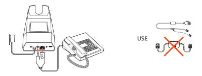
**IMPORTANT** Use configuration **A** on the bottom of the base, which works for most phones including Cisco phones.
