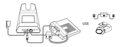
**IMPORTANT** *Cisco* phones use configuration **D** on the bottom of the base. Most other phones use the default configuration **A**.
