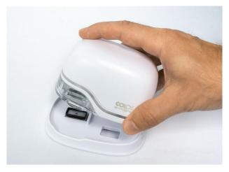
Fig. 23: Place into docking station
