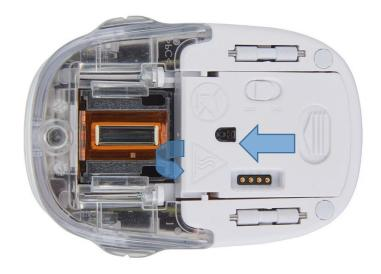
Fig. 43: Opening the sliding panel
