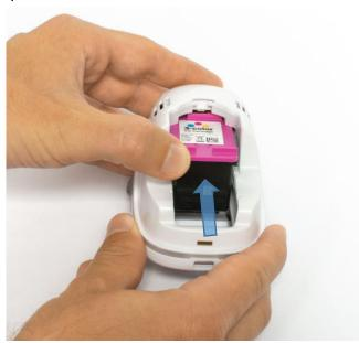
Fig. 13: Insert ink cartridge
