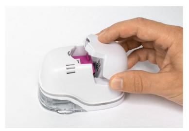
Fig. 15: Insert battery
