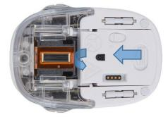
Fig. 11: Opening the sliding panel
