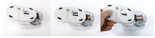
Fig. 29: Clean print head with wiper
