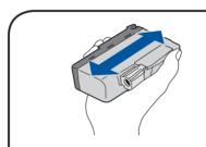
Quickly shake just the **black** ink cartridge horizontally 15 times as shown, before inserting it into the machine.
