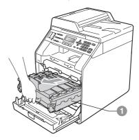
Gently pull the orange packing material towards the front of the machine to remove it.
