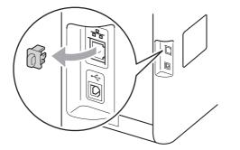
C Connect the network interface cable to the LAN connector and then connect it to a free port on your hub.
