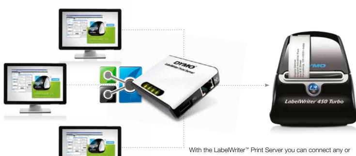
all (PC or Mac<sup>®</sup>) users on a network to a single LabelWriter™ label printer. It's e and a great way to provide customers the highest quality label printing at the lowest possible cost.
