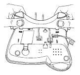
Hold the plinth as shown and push the lugs into the slots on the base until they click into place.
