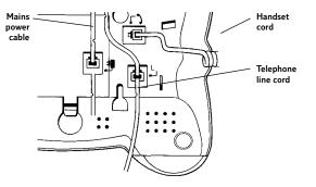
3. Route the cables as shown below for wall mounting or desk mounting.
