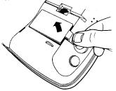
2. Lift the SIM card holder and slide card into it. Close the SIM card holder.
