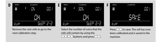
The calibration menu will now move to the next denomination. Repeat the process by selecting the desired denomination as shown above, or leave the calibration mode by pressing <u>cc</u>. If you want to switch to the next calibration item, use the <u>www</u> button.
