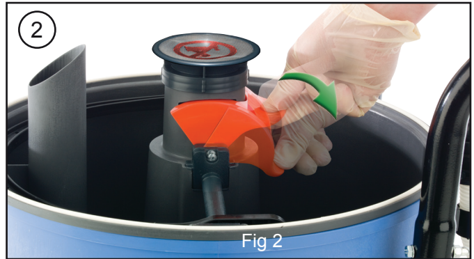
Remove the dome, unclip and remove the waste water tank (Fig 2)
