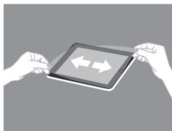
4. Apply slight pressure to the display so that the film lies down completely. Begin again on the long side.
